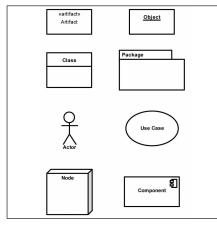
Fig. 2: Examples of UML Graphical Symbols
