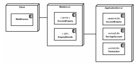
Fig. 11: A UML Deployment Diagram Representing Platforms, Networks and Components
